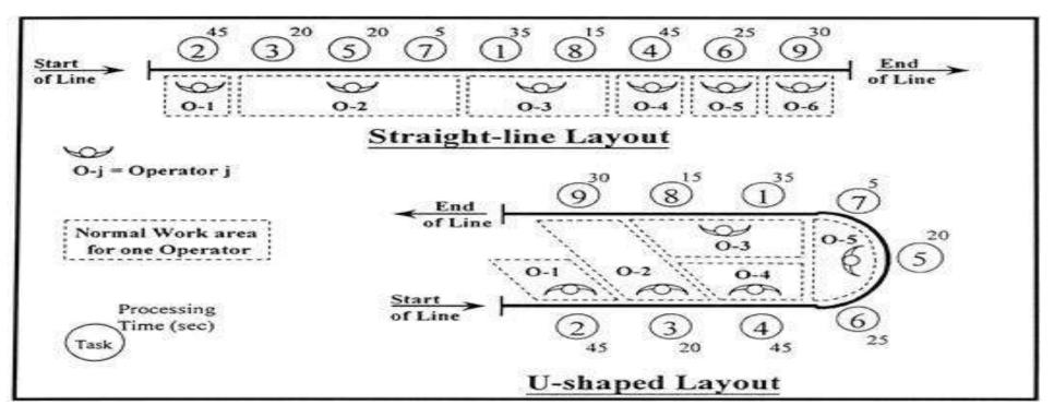
Figure: Product line or Assembly line layout (Line Processing Layouts)
